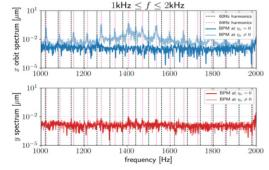
Figure 3: Horizontal (top) and vertical (bottom) orbit spectrum measured at 2 BPMs, one in a non-dispersive region (dark curve) and other in a dispersive region (light curve).
