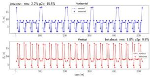
Figure 2: Measured betatron functions at BPMs after calibration of the linear optics with LOCO and of BPM offsets with BBA. Dots are measured values and lines are values from the nominal model.
