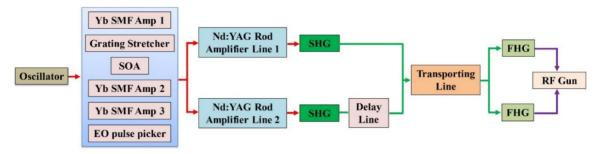
Figure 1: The layout of current Yb/Nd hybrid laser system for SuperKEKB commissioning.
