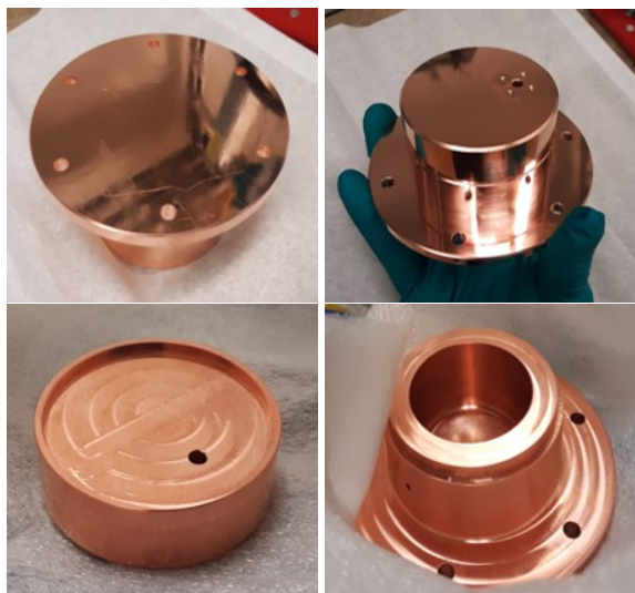
Figure 2: Brazed copper cavity (top) utilized in our cooldown tests and Q factor measurements. The Comeb cavity (bottom) will be tested in the near future.
