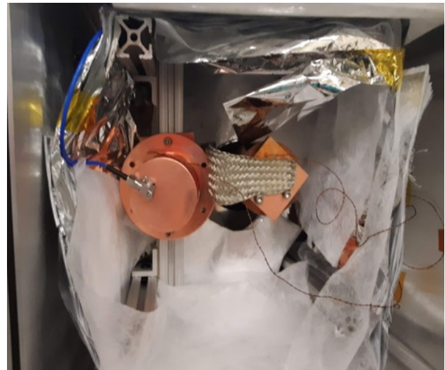
Figure 1: View of internal cryostat components, including MLI wrapping, 80/20 supports, coldhead, and thermal braid connection.
