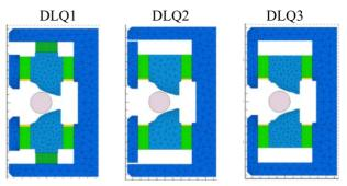
Figure 8: Cross sections of combined-function dipoles; thermal shims (yellow) are placed on top of the permanent magnets (green).
