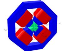
Figure 2: PQE quadrupole with coils (red), Vacoflux pole tips (green) and Armco yoke (blue).
