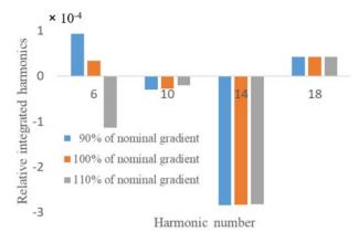
Figure 5: PQD relative integrated harmonics at 7.9 mm radius (63% of the aperture) at different excitation levels.
