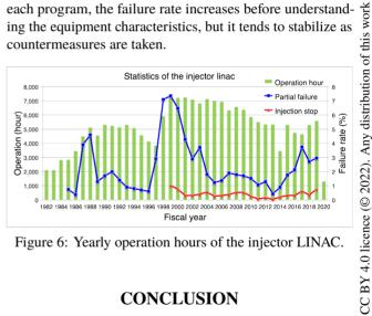
Figure 6: Yearly operation hours of the injector LINAC.
