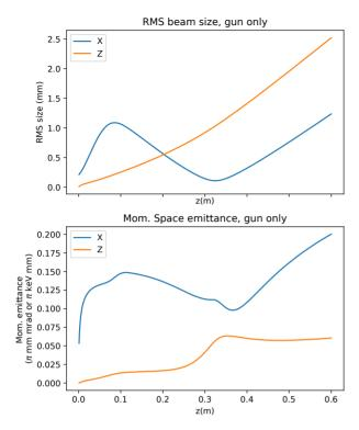
Figure 4: Gun only RMS and emittance development.
