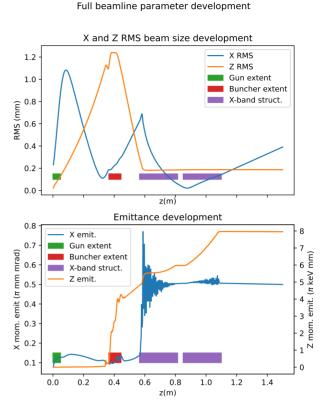
Figure 6: Development of bunch RMS and emittance through beamline.
