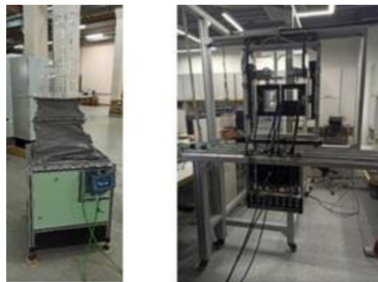
Figure 5: The positioning device for irradiated objects for SIMBO station (left) and the positioning system of the ISCRA station (right).
