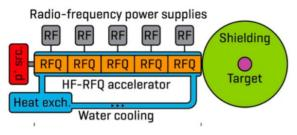
Figure 4: Scheme of the 7 MeV RFQ-based PET isotope production system.
