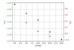
Figure 4: Focusing coefficients in the vertical plane  $M_{43}$ (green) and in the horizontal plane  $M_{21}$  (red) as a function of the tilt angle  $\gamma$  of the GaToroid isocentre side of the coil.
