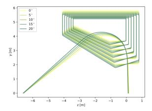
Figure 3: Configurations of the GaToroid coil for several isocentre-side angles  $\gamma$  (0 – 20°). Different configurations are shifted such that the beam arriving from the isocentre start experiencing the magnetic field at the same location. For each configuration a carbon ion beam of the same energy (300 MeV/u) is tracked such that it arrives with minimum angle to the same isocentre.
