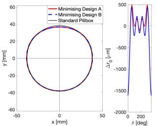
Figure 3: Comparison of the physical dimensions of the cross-sections of the three different designs (left) and the deviation of Minimising Design A [red] and Minimising Design B [blue] from the Standard Pillbox radius (right).
