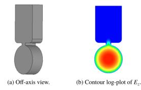
Figure 1: Pillbox cavity coupled to an RF input port via a single-slot that supports a 3 GHz fundamental accelerating mode.
