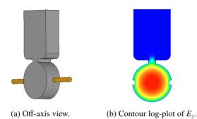
Figure 2: Pillbox structure oversized by 100  $\mu$ m that supports a fundamental accelerating mode tuned to 3 GHz by two, one-way tuning pins.  $E_z$  is plotted at the longitudinal centre of the structure.
