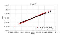
Figure 6: Plot of the Y' versus Y phase space plot for an ensemble of rays tracked through B-C-B triplet comparing results with and without the dipole excitation considered.
