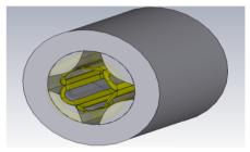
Figure 1: 3D model of FSQC's Sextupole nested inside of the quad iron yoke in CST Studio Suite<sup>®</sup>.
