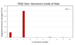
Figure 2: Integrated harmonic decomposition analysis of FSQC Sextupole with inclusion of quadrupole iron yoke [1,2]. Reference radius of analysis is R=8.1cm from beam axis.
