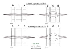
Figure 3: Optics simulation of triplet with a beam rigidity of 8 Tm. The top 2 images are without the inclusion of the dipole harmonic term. The bottom images are the same calculation with the inclusion of the dipole harmonic term. Images in the right column are the dispersive plane and images in left column are the non-dispersive plane. The ray limits refer to the position and momentum range of the ensemble of rays tracked. Letter labelling refers to the corresponding FSQ magnet.
