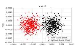
Figure 4: Plot of the X versus Y position for an ensemble of rays tracked through B-C-B triplet comparing results with and without the dipole excitation considered.
