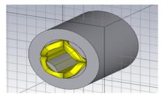
Figure 10: Picture of FSQC quad and iron yoke 3D model in CST Studio Suite<sup>®</sup>. Quad coils are each 0.9 m in length and the iron yoke is 0.7 m in length.
