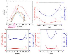
Figure 6: The DA observed at the injection point with  $\beta_{0x} = 20.0 m$  and  $\beta_{0y} = 2.3 m$  (left-upper), chromaticity (right-upper) and ADTS (bottom). In the figure of DA, the dashed line is for the ideal ring and the solid lines are for the ring with sextupole misalignment (rms 25  $\mu m$ , max.  $\pm 50 \ \mu m$ ).
