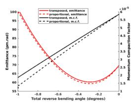
Figure 2: Evolution of the emittance and the momentum compaction factor (m.c.f.) with the total reverse bending angle, for the two methods of angle restoration.
