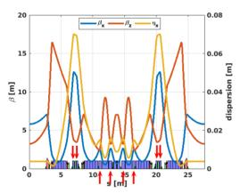
Figure 1: Location of the reverse bends (red arrows) in the lattice. All dipoles are represented in blue.
