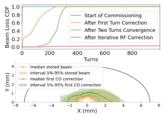
Figure 2: (TOP) Beam loss cumulative distribution as a function of the number of turns for 30 rings. (BOTTOM) Dynamic aperture during *on-axis* injection before BBA. Physical aperture is shown in black.
