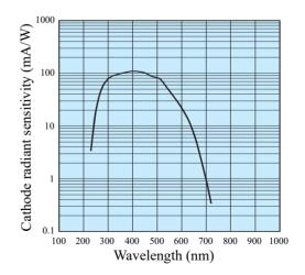
Figure 1: Cathode sensitivity for PMT [6].
