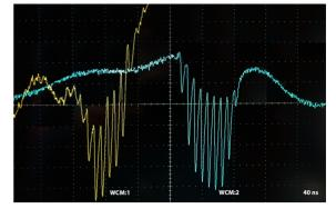
Figure 6: Wall current monitor signal at the HBT upstream (yellow) and downstream (green).
