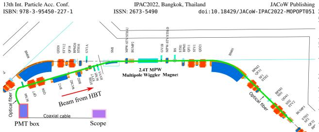
Figure 2: Schematic view of the optical fiber (green line) installation section.
