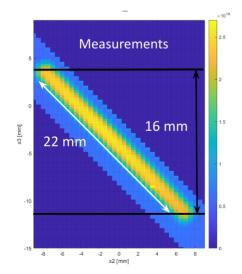
Figure 1: Measured gas jet profile on BGCv3 at CERN.
