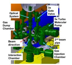
Figure 4: 3D model BGCv4 integrated in the HEL.
