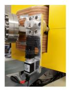
Figure 2: The experimental setup of the CCD camera in the booster.
