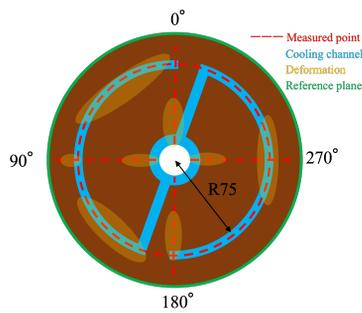
Figure 8: A schematic diagram of the pressure test.
