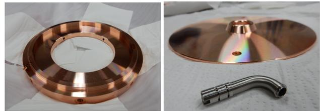
Figure 11: Photo of disk (left), washer, and stem (right) for the first tank.
