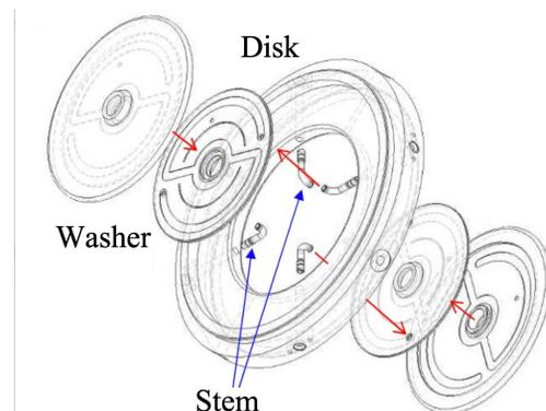
Figure 2: Configuration of prototype cell.
