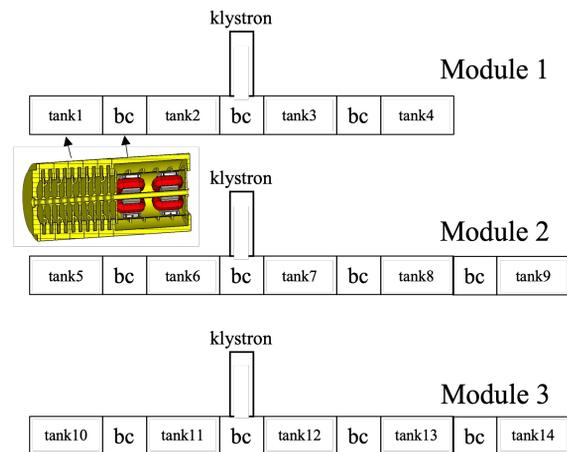
Figure 1: The configuration of the muon DAW. Schematic of the entire accelerator and 3D model of the 1st tank with bc is shown.
