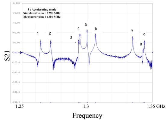
Figure 10: A example of frequency measurement result with the prototype cell.
