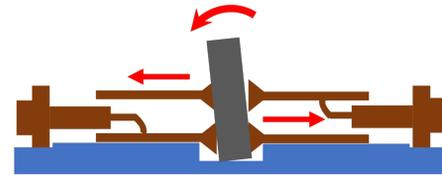
Figure 6: Schematic diagram of causes of parallelism and concentricity deterioration. The gap between the positioning jig and washer causes the jig to tilt, which in turn causes the upper washer to shift significantly and the lower washer to shift as a result.
