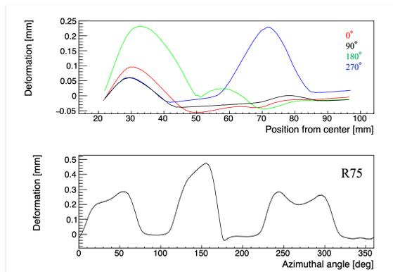
Figure 9: The deformation measured by the pressure test.
