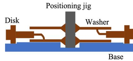
Figure 3: The configuration for brazing.
