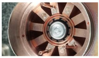
Figure 2a: Picture showing 10 cavities, straps, and antenna posts attached to the vanes of the anode body.
