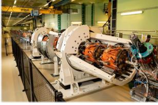
Figure 2: World-wide first rotator system (white structure) in the high energy beam transfer line. Seven quadrupoles (orange) are mounted on the structure and rotated synchronously with the gantry located downstream. With a rotator, the beam parameters at the gantry isocenter become independent from the gantry rotation angle.
