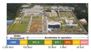
Figure 1: Layout of the 100 MeV proton linac at KOMAC and upgrade plan.
