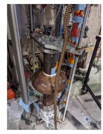
Figure 1: SN 38-39 cavity on the RF testing insert under vacuum.
