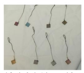
Figure 1: Samples after chemical treatments, before coating.
