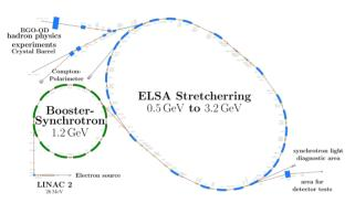
Figure 1: The Electron Stretcher Facility ELSA.
