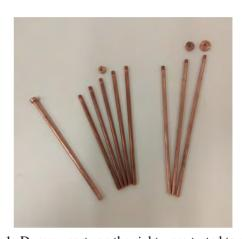
Figure 1: Dummy parts on the right were tested to achieve critical coupling strength at room temperature. Center dummy components are of similar dimensions to the previously installed coupler on the left and were used to determine the required length adjustment.
