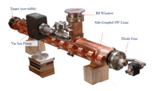
Figure 1: SAMEER made 15 MeV linac tube.
