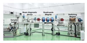
Figure 1: The current setup of R&D beam line consists of a five-port switching magnet, a set of quadrupole magnets, a beam diagnostic device and a sample holder.
