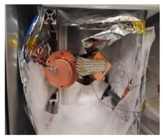
Figure 1: View of internal cryostat components, including MLI wrapping, 80/20 supports, coldhead, and thermal braid connection.
