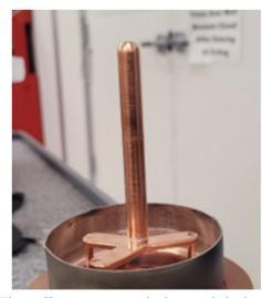
Figure 2b: Antenna attached to anode body.
