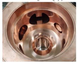
Figure 2: Inner view of the cavity body. Courtesy of VITZTRO TECH.
