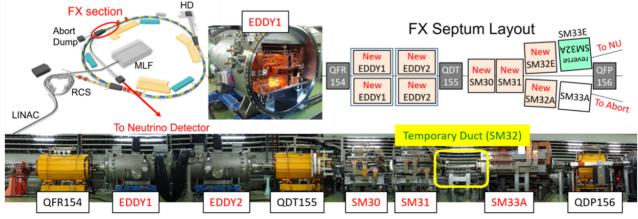
Figure 1: Pictures and schematic layout of the fast extraction septum magnets.
