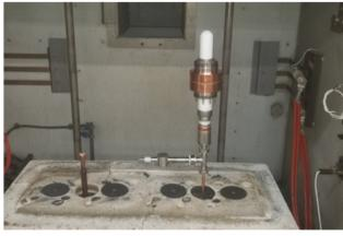
Figure 1: The prototype 1497 MHz magnetron in the bakeout oven at RELL, showing the ion pump used for conditioning.
