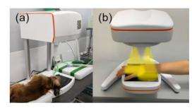
Figure 1: Adaptix (a) veterinary and (b) extremity DT systems. Reproduced with permission from Adaptix Ltd.
