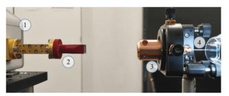
Figure 1: Experimental setup. (1) Extender waveguide port (2) Horn antenna (3) Integrated horn-waveguide structure (4) Movable obstacle. Reproduced from Ref. [16]
