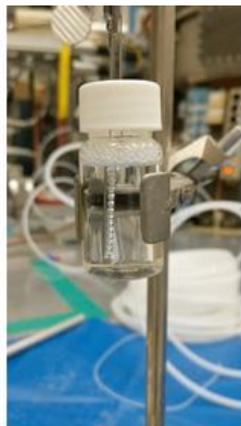
Bismuth oxide target Capturing ^{211}\text{Rn} gas
