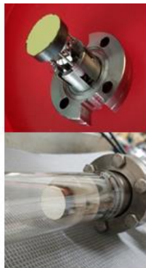
Bismuth oxide target Capturing ^{211}\text{Rn} gas
