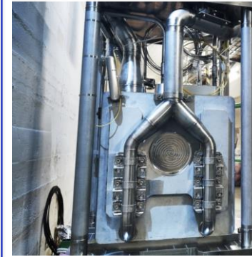
Third-generation n_TOF target before installation in the beamline.
