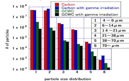
Figure 5: Measurement results of the size and number of the dust particles generated.
