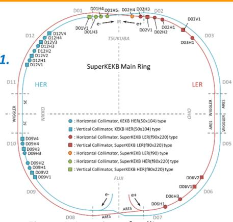
Figure 1: Location of collimators in the main ring of SuperKEKB.
