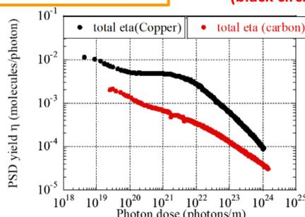
Figure 2: Comparison between PSD of copper and carbon.
