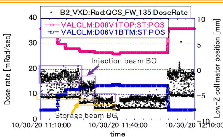
Figure 8: Measured value of BG when the gap of low-Z collimator changed.
