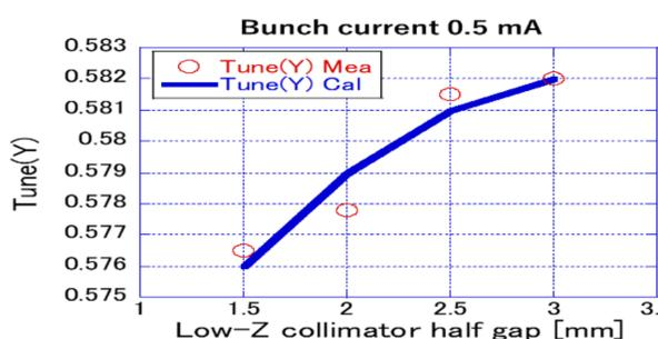
Figure 10: Measured tune shift compared with the estimated values from calculated impedance.
