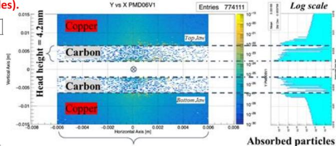
Figure 3: Absorbed particle distribution at the D06V1 jaw attached carbon (L = 60 mm).
