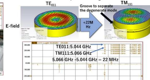
Figure 7: Excited mode in the cavity.
