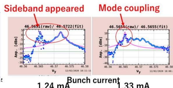
Figure 11: Observation of TMCI phenomenon (0 mode and -1 mode coupling)
