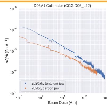
Figure 9:  $dP/dI$  beside the low-Z collimator as a function of the beam dose.
