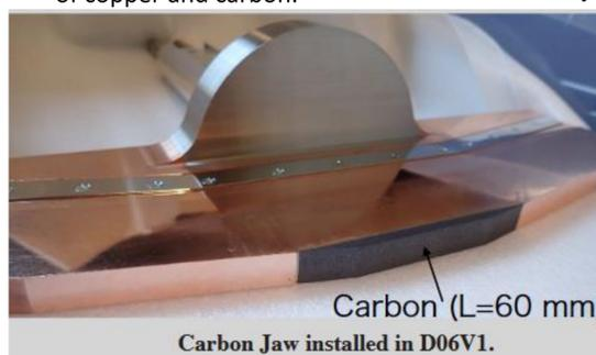
Figure 4: The jaw attached carbon
