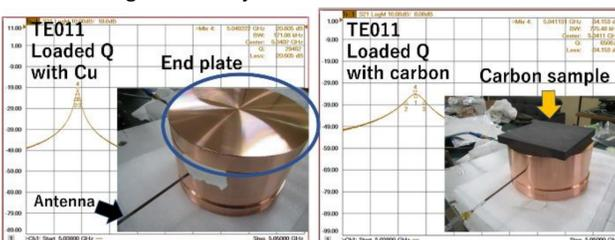
Figure 6: Cavity for measurement of electronic conductivity of the sample.
