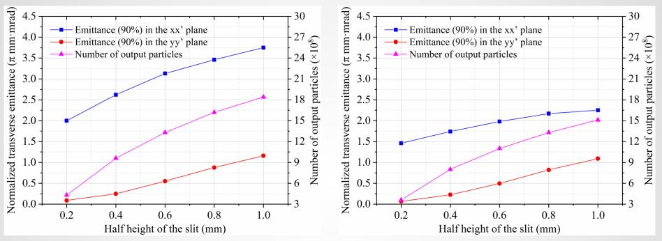
Output particle number and transverse emittances on the half height of the slit. The half width of the slit in the horizontal direction is 6 mm (left) and 4 mm (right)
