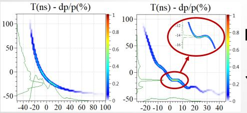
□ Energy spread compression with debuncher (700 kV, 80 MHz)
