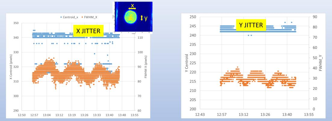
The beam was jittering and there was no clear position drift recorded. But it is clearly showing that the beam size was swinging with time at about 15 minutes per cycle.
