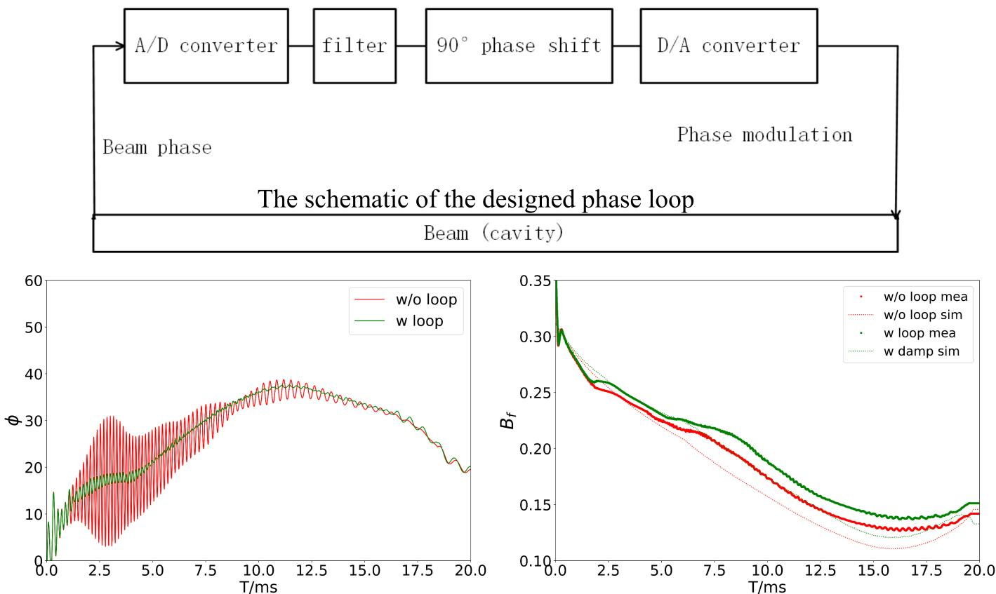
The beam phase oscillation is also damped by the optimized loop. The measured bunch factor is also same with that without the loop. The transmission efficiency is also maintained, but a little proton loses in the arc section when the loop with fast damping rate.
