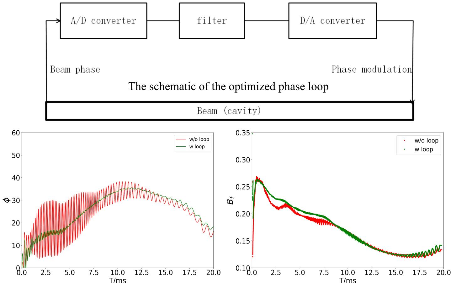
The beam phase and the bunch factor with and without the designed loop.
