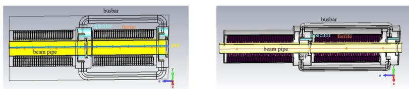
The CST simulation mode of the cavity prototype (left) and cavity (right)
