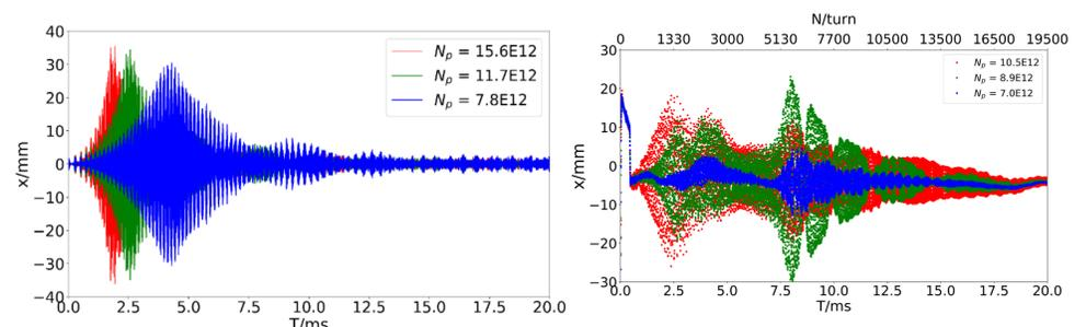
The beam position driven by the cavity impedance (left) and measurement (right)
