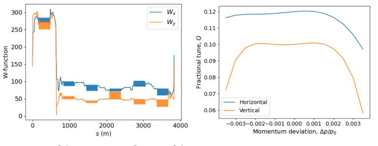
$$b = rac{1}{eta} rac{\partial eta}{\partial \delta} \qquad \qquad a = rac{\partial lpha}{\partial \delta} - rac{lpha}{eta} rac{\partial eta}{\partial \delta}$$
