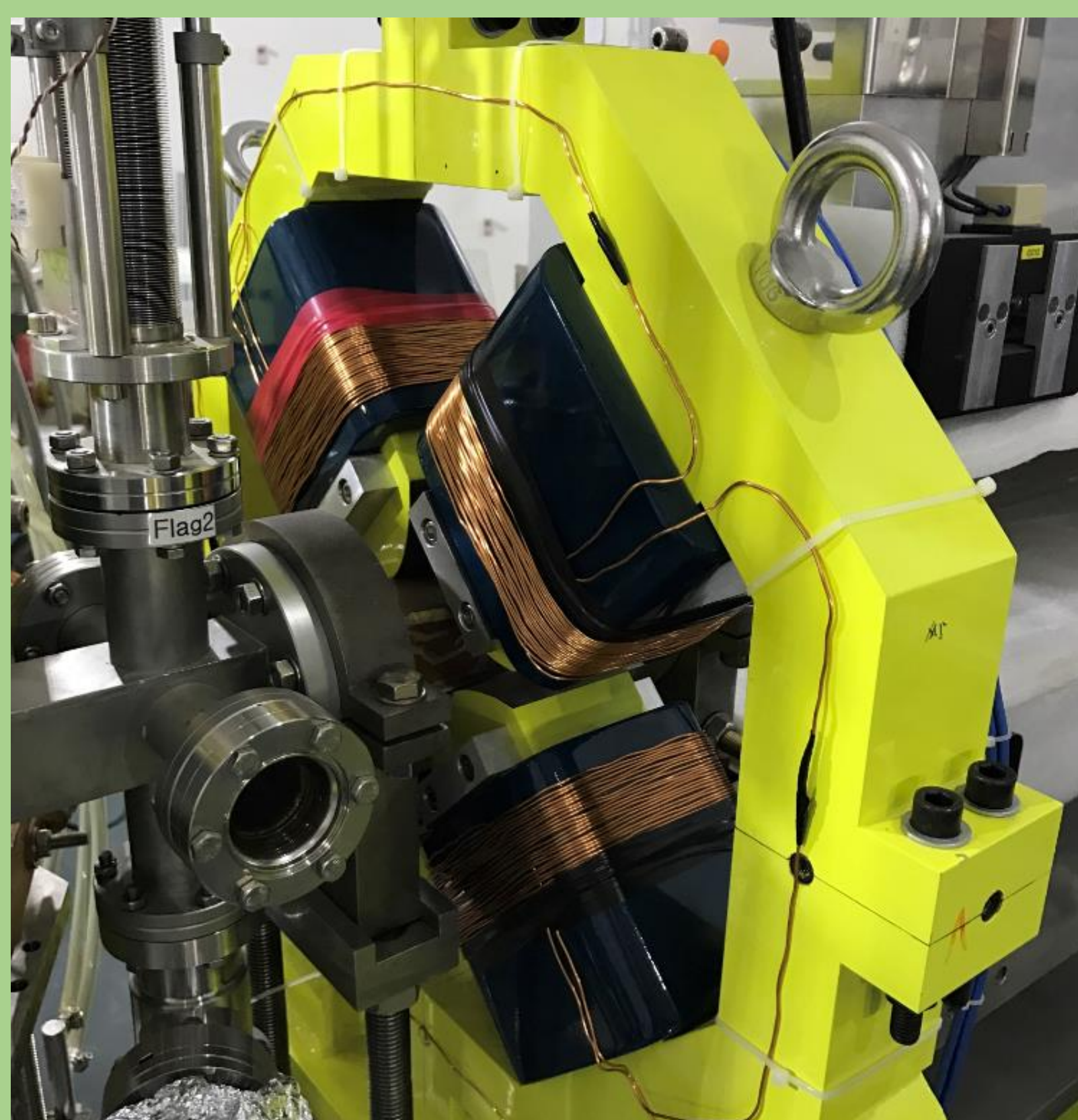
Fig. 2 Vertical steering coil S3 wound on Q5.
