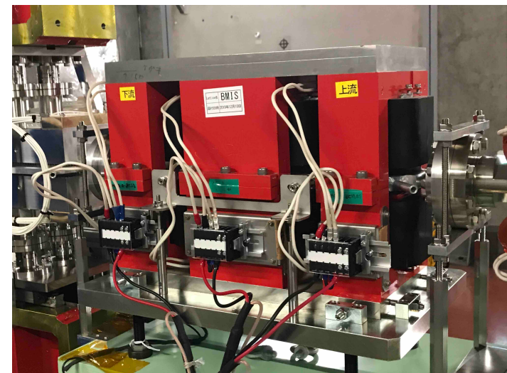
Chicane magnet installed in the cERL
