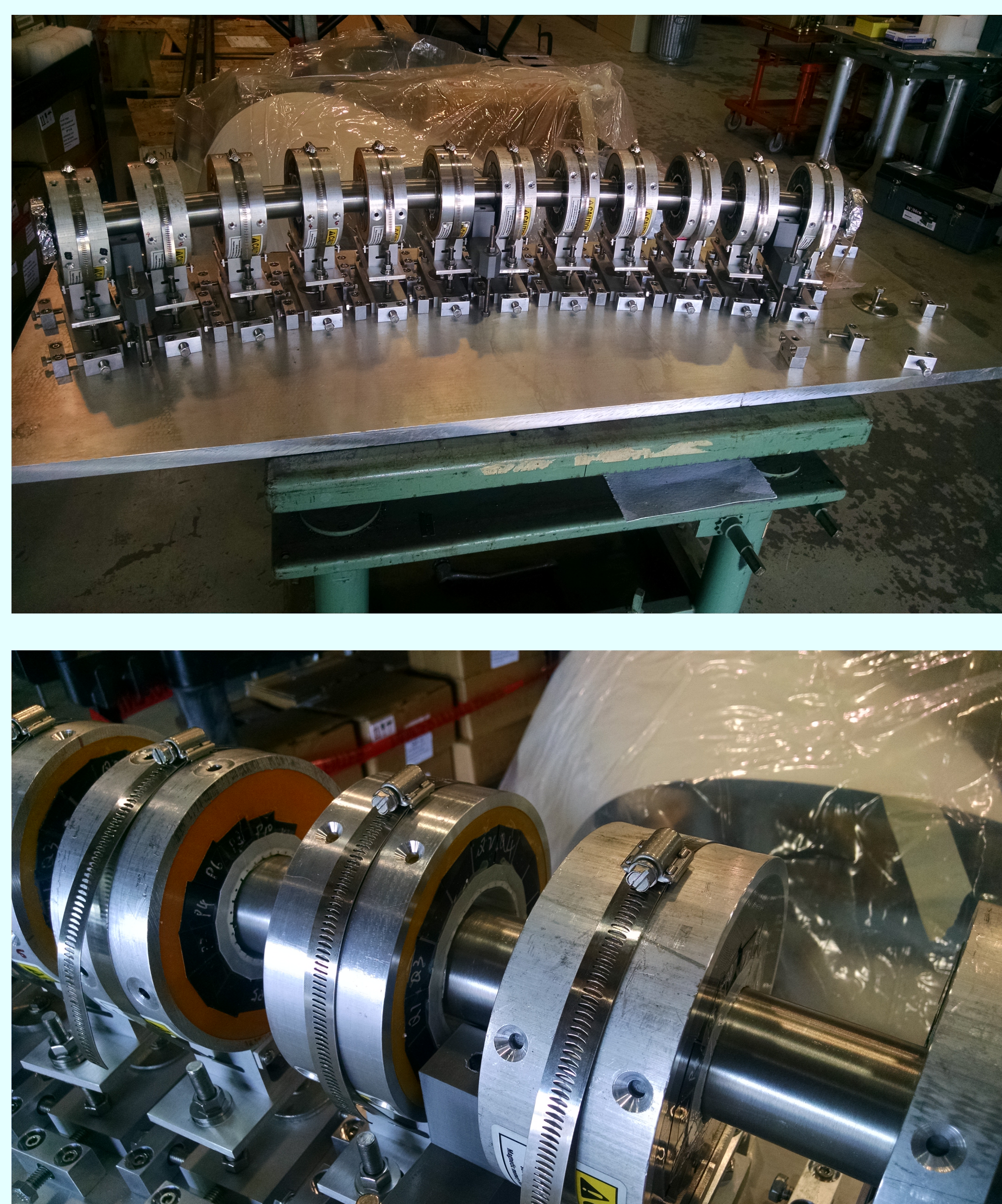
Figure 2: NS-FFAG with 12-magnet girder at BNL Advanced Test Facility.
