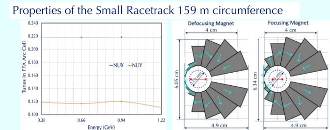
**Figure 10:** Tune dependence on energy in the FFA small racetrack arc within the energy range between  $0.38 < \Delta E < 1.22 \text{ GeV}$ .
