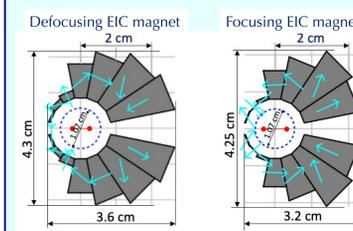
**Figure 7:** Good field @  $R_{BD}=5.33 \text{ mm}$  maximum orbit offsets @  $B_D$ :  $2.28 \text{ mm} < \Delta x_{MAX} < 2.52 \text{ mm}$ , maximum field of  $B_{D,MAX}=0.363 \text{ T}$
