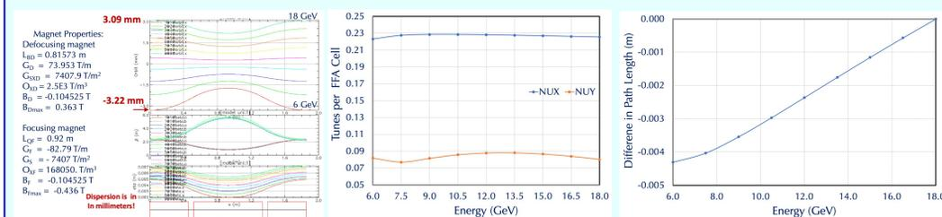
**Figure 5:** The Main FFA-LG arc cell properties with maximum orbit offsets  $-3.09 \text{ mm} < x_{MAX} < 3.22 \text{ mm}$  with combined function permanent magnets.
