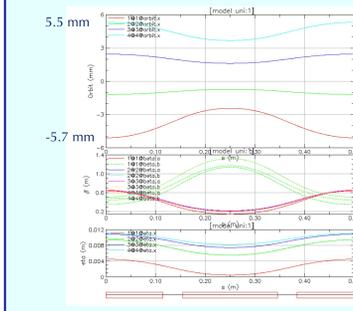
**Figure 9:** Lattice functions and orbits in the single arc cell of the small 159m racetrack with the permanent combined function magnet properties. Maximum orbit offsets in  $Q_x$ :  $-5.7 \text{ mm} < \Delta x_{MAX} < 5.5 \text{ mm}$  or in  $Q_y$ :  $-3.7 \text{ mm} < \Delta x_{MAX} < 4.4 \text{ mm}$
