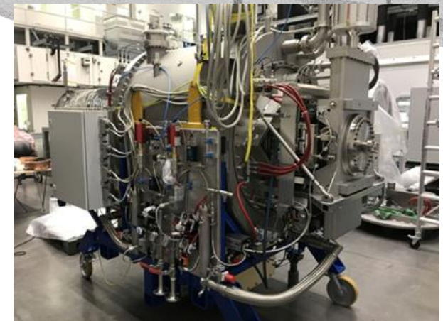
First Sirius SC cavity cryomodule
