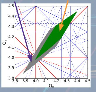
A double harmonic RF bucket with the higher harmonic in anti-phase gives bunch lengthening. Longer bunches have a lower line density, which leads to reduced tune spread. The smaller tune footprint allows some resonance lines to be avoided, reducing the risk of losses and/or emittance growth.
