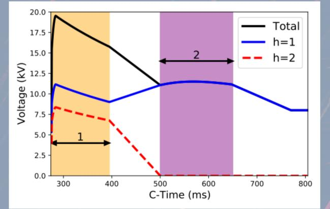
This beam requires high brightness and a large longitudinal emittance. Bunch lengthening at the start will reduce the impact of space charge, then phase noise will be applied for controlled longitudinal emittance blow-up.
