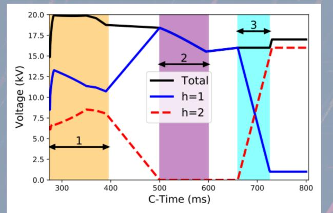
This the only cycle where two bunches are extracted. Longitudinal splitting is done as late in the cycle as possible as accelerating in h=1 is easier, but must not be too late or there may be a microwave instability.
