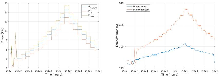
$\Delta T/\Delta P_{in}$ =0.78 K/kW in SW regime. Here, fields at maximum doubled compared to TW regime  $\rightarrow$  corresponds to four times the power level IR window warmer than in full power TW, but still within tolerances A scan of different reflective end distances should be studied (phase shifter), but what SW regime establishes in the FPC?
