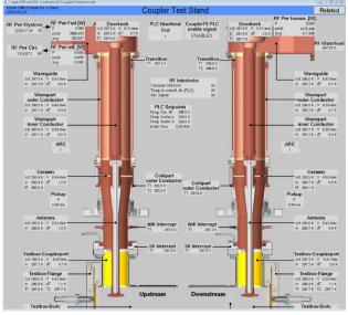
Epics panel with a selection of sensors (missing water flow et al.)
