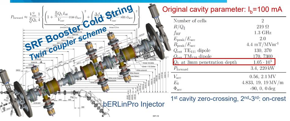
Current reduction from 100 to 6 mA  $\rightarrow$  FPC retracted by 20 mm to Q<sub>L</sub>=1.74 ·10<sup>6</sup>  $\rightarrow$  Forward power per coupler: <u>7 kW in TW</u> and <u>1.7 kW SW (original 120 kW TW and 25 SW)</u>
