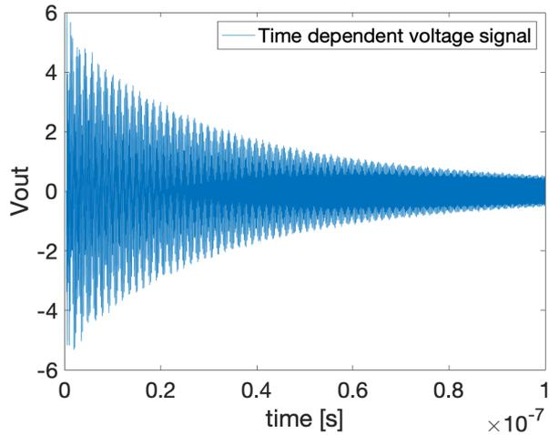
Output voltage signal coming out of one of the coaxial ports for position cavity.
