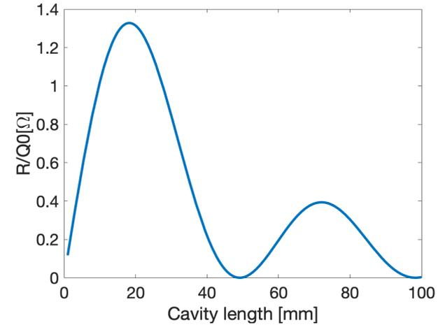
Dependence of the shunt impedance on the cavity length.
