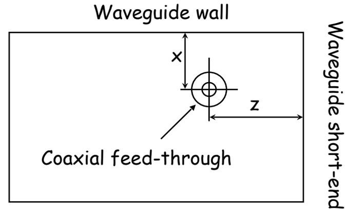
Exposition of how sufficient transition is achieved between the waveguide and coaxial antenna by changing the  $x$  and  $z$  parameters.
