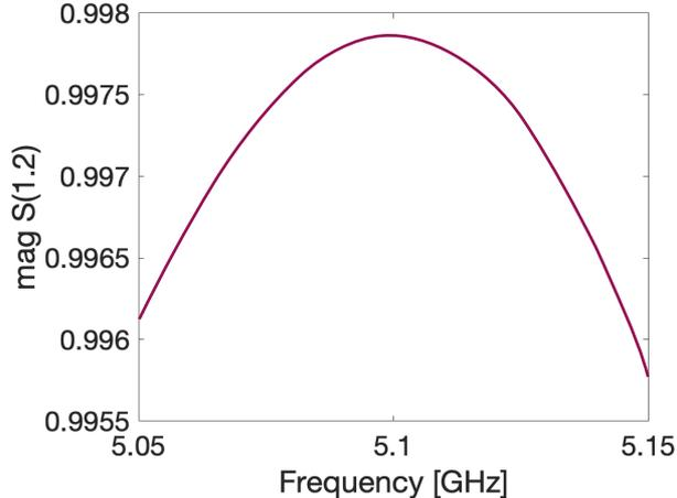
Mag S(1,2) parameter for 5.1 GHz waveguide to coaxial transition for the direct coupling case.
