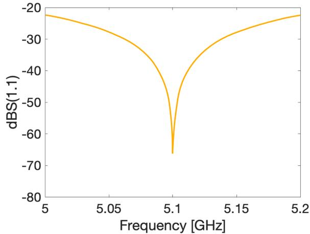
dB S(1,1) parameter for 5.1 GHz waveguide to coaxial transition for the direct coupling with whip antenna.
