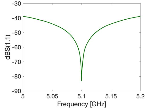
dB S(1,1) parameter for 5.1 GHz waveguide to coaxial transition for the capacitive coupling.
