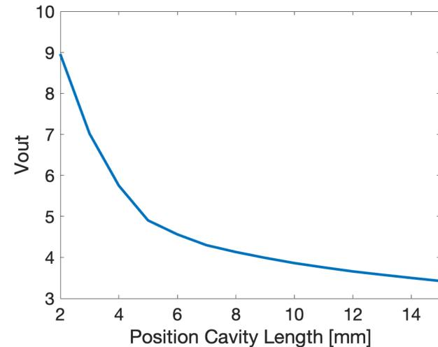
Output voltage  $V_{out}$  dependence on the position cavity length variation.
