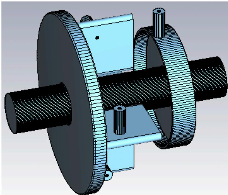
Cavity BPM pickup schematic view (shown: vacuum).
