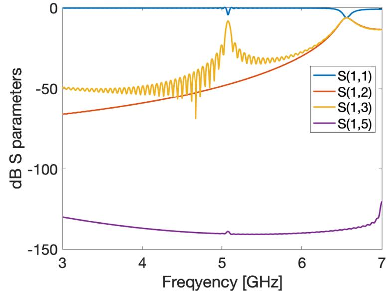
Position cavity ports cross-coupling and isolation between the position and reference cavities.
