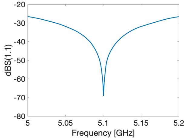
dB S(1,1) parameter for 5.1 GHz waveguide to coaxial transition for the inductive coupling with whip antenna.
