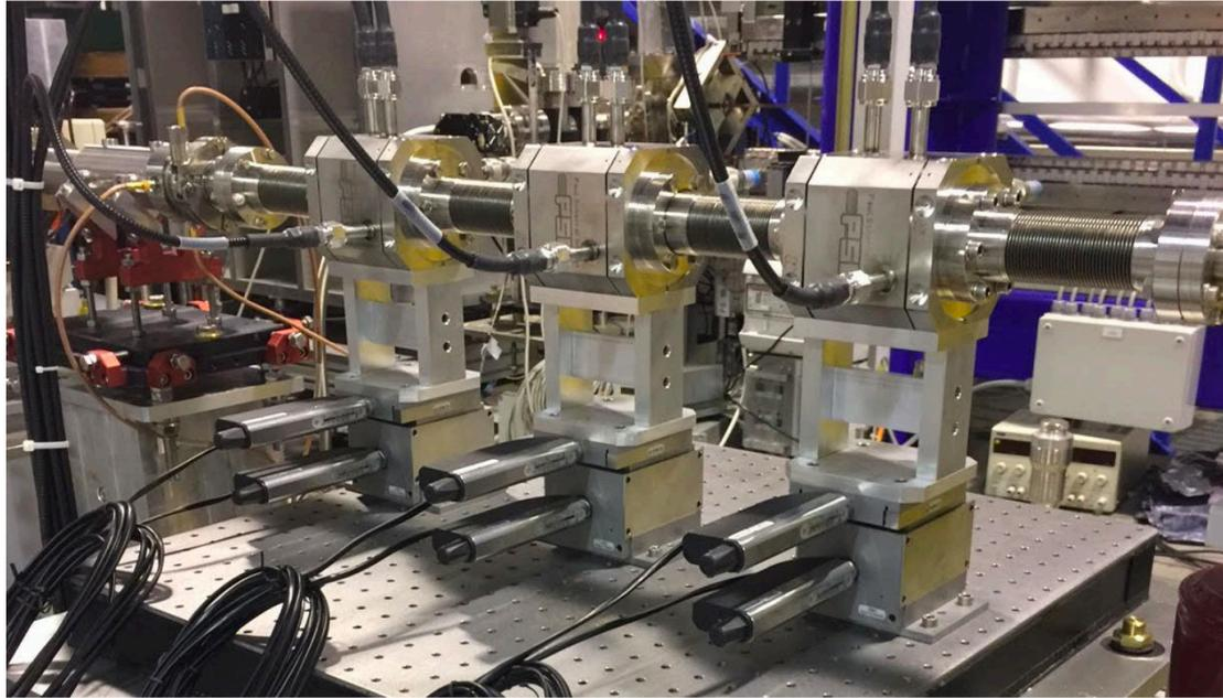
Once the first prototypes will be fabricated, bench-top measurements and beam tests will be performed. Such a new test-bench for cBPMs at SPARC-LAB at INFN-LNF was designed and will be used in the prototype tests.
