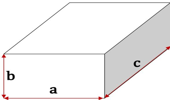
The width of waveguide (a) has to be chosen such, that its cut-off frequency is located between TM<sub>010</sub> and TM<sub>110</sub> cavity modes.
