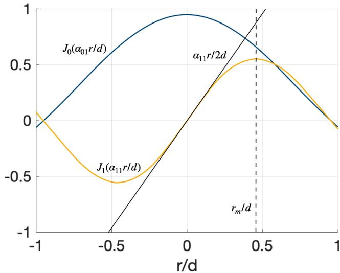
$$\frac{R}{Q_{110}} = \frac{V_{110}^2(r_m)}{2\omega_{110}W_{110}} = \frac{2Z_0 l J_{1max}^2 T_{ir}^2}{\pi \alpha_{11} d J_0^2(\alpha_{11})}$$
