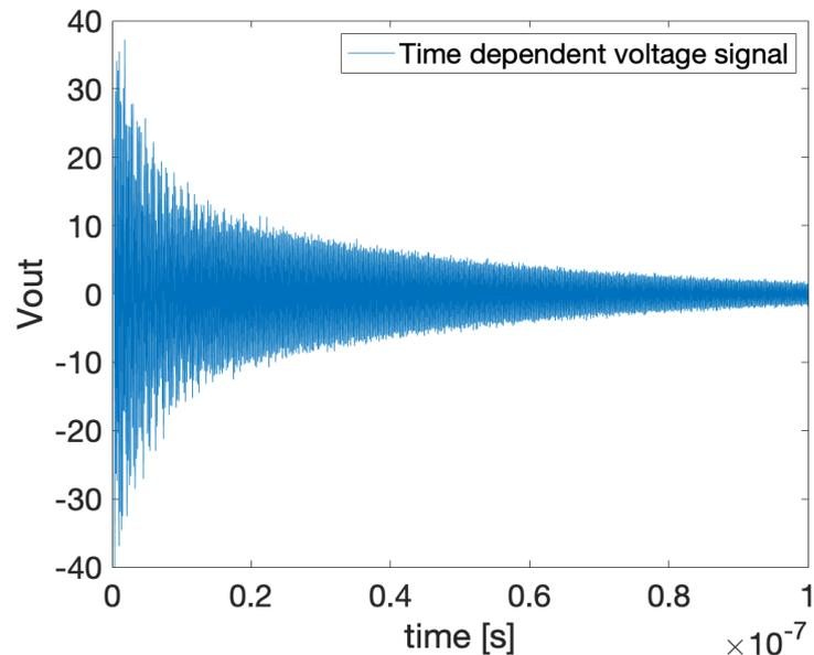
Output voltage signal coming out from the reference cavity with a 1 mm beam offset. Wakefield simulation.
