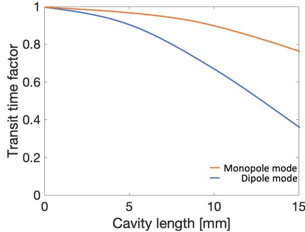
Transit time factor for the monopole and dipole modes of a pillbox cavity with different lengths.
