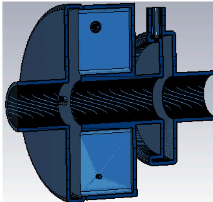
Cavity BPM pickup half-cut schematic view (shown: copper shell).
