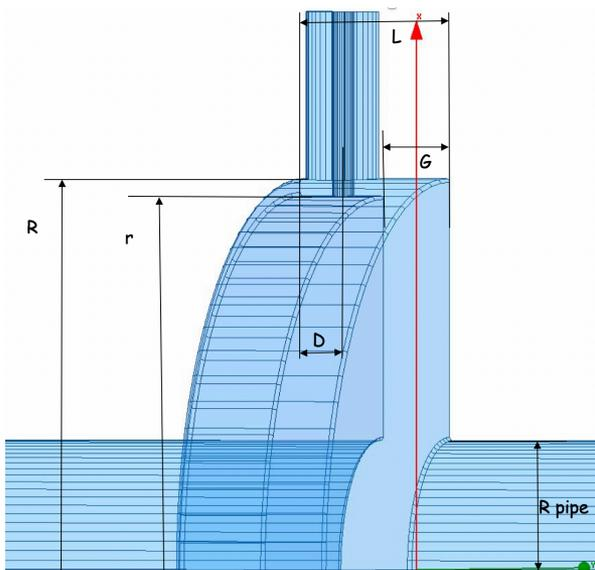
Schematic view of reference cavity with geometrical indications.
