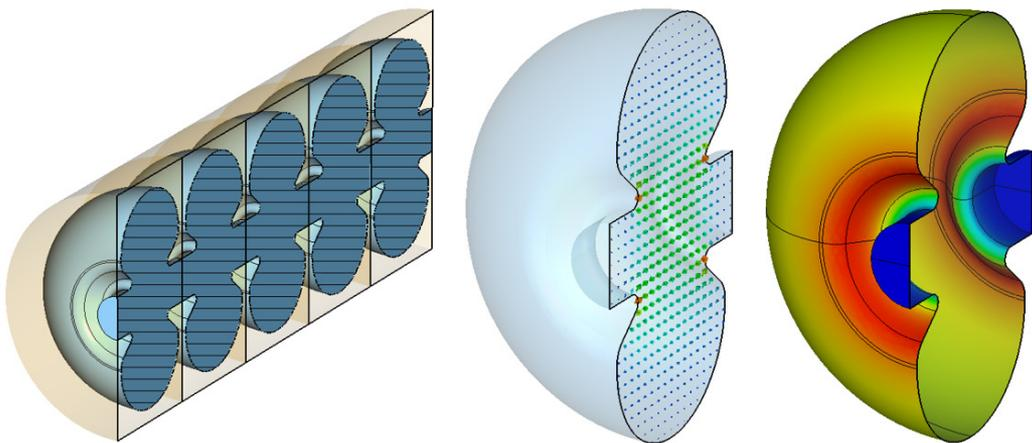
S-band structure for  $\beta=0.84$ : 5-cell structure section (left); electric field within a cell; current distribution on the cell inner surface.
