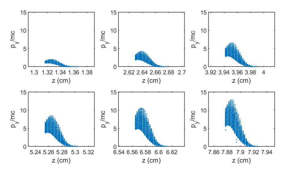
Bunch particles dynamics in the  $p_y/mc - z$  plane in the case of off-axis injection
