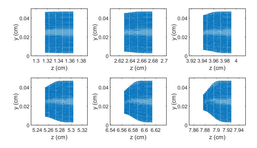
Dynamics of the off-axis bunch on the y – z plane. Vertical axis limits correspond to half of plasma channel width, horizontal axis limits correspond to the frame around the bunch. The initial vertical offset of the bunch is 0.25 mm, the length of the structure is 8 cm.
