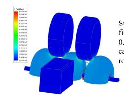
Surface magnetic fields with peak of 0.85 MA/m, calculated with fillet rounding of 0.1 mm
