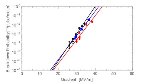
When we compare structure with the same Epeak/Eacc <sup>3SW</sup> A1.5 T3.03 Braz Euclid and wildly different Hmax\*Z05trace.5 (T3.03 BH2 EState-1400 ns coupled vs 1.1 in on-axis coupled), we see that peak magnetic field or associated with it peak pulse surface heating is much better predicator of breakdown rates than the peak surface electric field.
