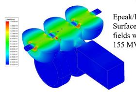
Epeak/Eacc = 2.65, Surface electric fields with peak of 155 MV/m@1MW.
