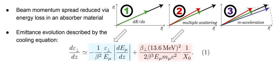
• Cooling performance increased by using low Z, high radiation length materials and tightly focusing the beam at the absorber (low  $\beta_{\perp}$ )
