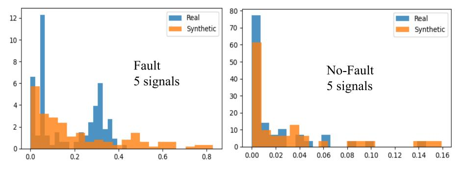
→ Lower magnitude of combined signal during fault (left), higher values obtained during normal times (right)
