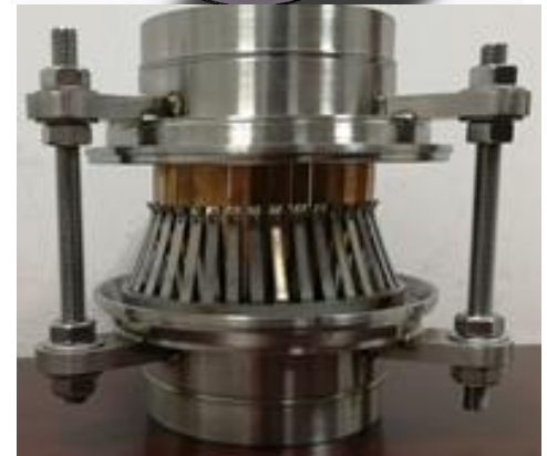
Assembled of contact and spring fingers
