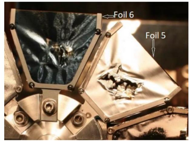
Foil 6 was coated with carbon. These foils were replaced after the high intensity operation at 5.75GeV.
