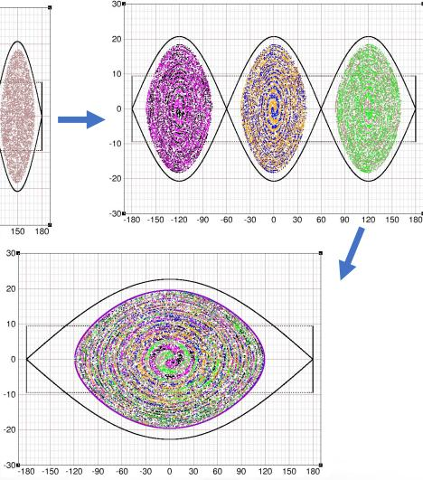
Initial six Au77+ bunches to be merged. Total emittance of 6 bunches is 0.60 eV-s per nucleon.
