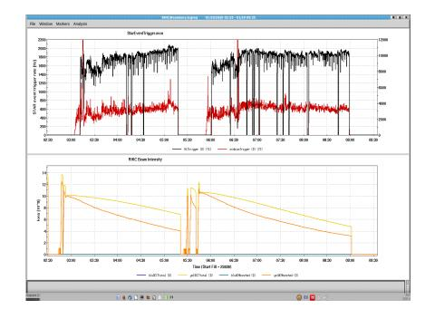
The upper plot shows the fixed target event rate (in black) and min-bias rate (in red) over the time period of twophysics stores at 9.8 GeV. The lower plot shows the beam intensity evolution during the stores, total beam intensity inlight yellow and bunched beam intensity in dark yellow.
