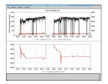
Vertica orbit bump implemented during the fixed target stores to maintain the experimental rates.
