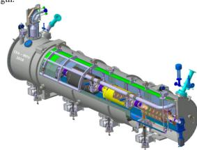
Figure 1: ESS medium-beta cryomodule general layout.
