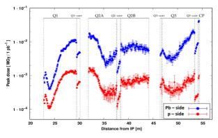
Figure 2: Peak dose profile in the inner coils of the triplet as a function of the distance from the IP, induced by Pb-p collisions on the *Pb-side* (blue) and the *p-side* (red). Values are normalized to a reference integrated luminosity of 1  $pb^{-1}$ .
