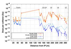
Figure 3: BLM pattern along the LSS on the right side of IP1, as measured during the indicated Pb-p (orange) and p-Pb (light blue) physics fills and simulated with FLUKA (red and blue, respectively). Experimental doses are divided by the product of the fill luminosity and the 2.11 b INI cross section value.
