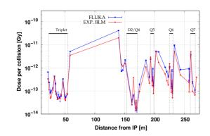
Figure 4: BLM pattern along the LSS on the right side of IP1, as measured during the Pb-Pb physics fill #7473 in 2018 and simulated with FLUKA. Experimental doses are divided by the product of the fill luminosity and the 438 b cross section value, corresponding to the sum of the INI and EMD cross sections.
