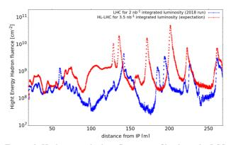
Figure 6: High energy hadron fluence profile along the LSS on the right of IP1 as induced by Pb-Pb collisions in the HL-LHC (red) and LHC (blue) configuration. Values averaged over a 40 cm horizontal interval centred on the machine axis and a 20 cm vertical interval centred 30 cm from the floor level. They are normalized to an annual integrated luminosity of  $3.5 \text{ nb}^{-1}$  and  $2 \text{ nb}^{-1}$ , respectively. INI and EMD contributions are added up according to their cross sections.
