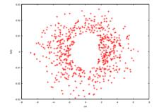
Figure 4: RCS lattice Phase space plot of dp/p and cm showing lost particles over 200 turns.
