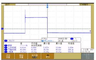
Figure 8: Parament of the pulse-forming circuit.
