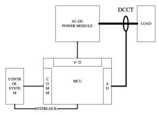
Figure 2: Unipolar DC power supply.
