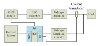
Figure 11: Conceptual of high voltage PS.
