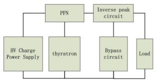
Figure 9: Linear modulator.
