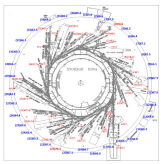
Figure 1: Hand held noise meter mapping.
