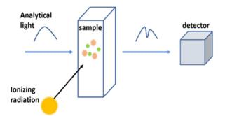
Figure 1: Schematic of pulse radiolysis.
