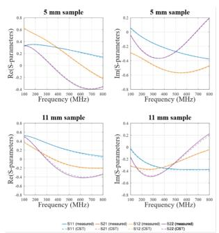
Figure 4: S-Parameters, measured field (solid lines) compared with CST simulated model.
