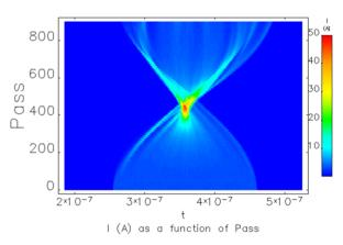
Figure 3: Simulated beam instabilities with ELEGANT.
